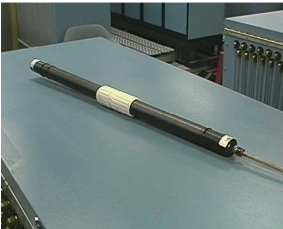
Figure 3 – Coupler Installed with Duct and Ready for Pressure Testing
