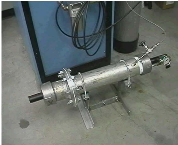
Figure 5 – Water Tightness Test Apparatus with Specimen Under Test Conditions
