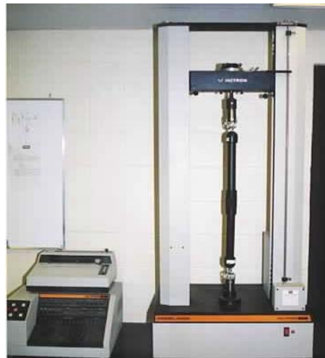
Figure 7 – Pull Out Resistance Tensile Test
